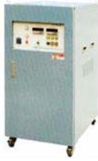
electricity which is transferred via a semiconductor switch into the coil in a few milliseconds. The magnetic field strength needed for the sintered Nd-Fe-B magnets is 2400 kA/m. We also deliver unmagnetized magnets if needed.
