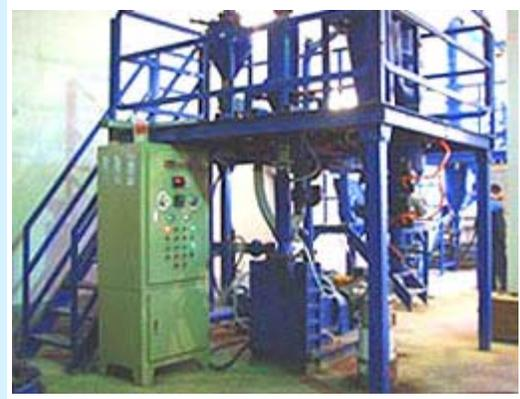
②Coarse crushing machine, Mid-crushing Machine
